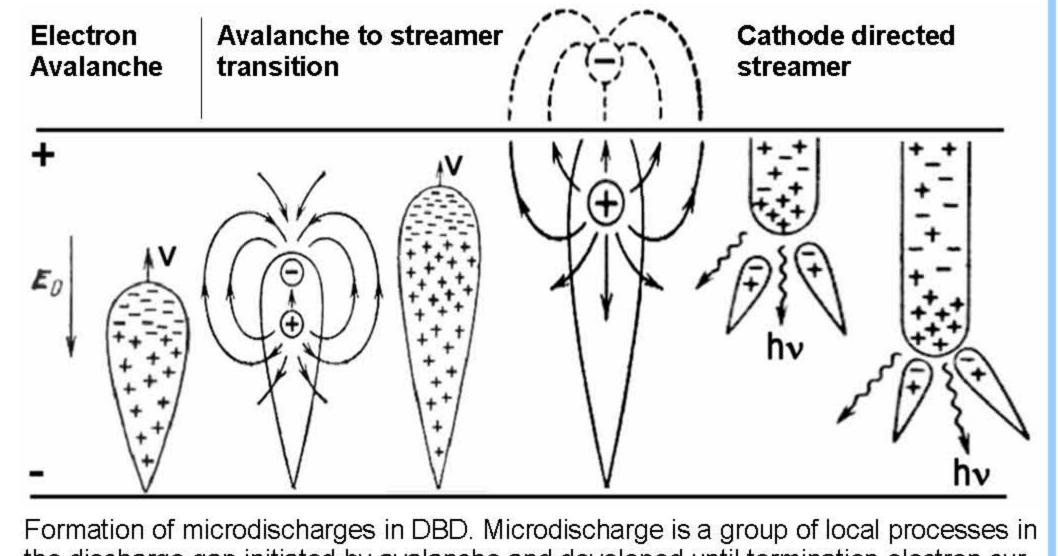
the discharge gap initiated by avalanche and developed until termination electron current. Typical microdischarge parameters in air 1 atm. presented in table below.
